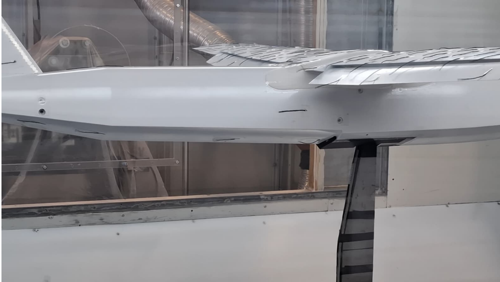
Figure 5.19: Flow visualization behind the step ( \alpha = 0^\circ , \beta = 0^\circ , flaps 20^\circ )
