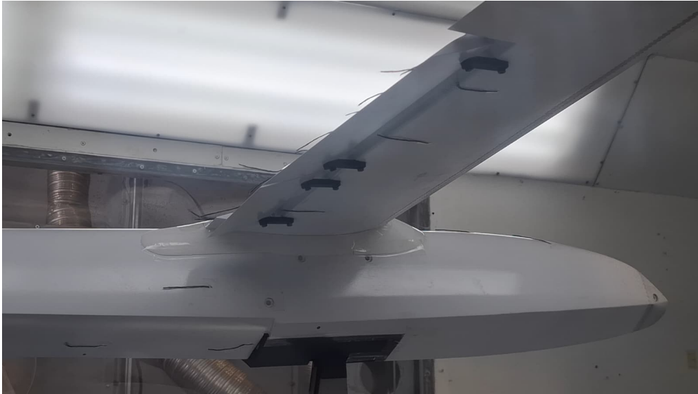
Figure 5.20: Tufts bending towards the slot of the flaps (flaps 20°)
