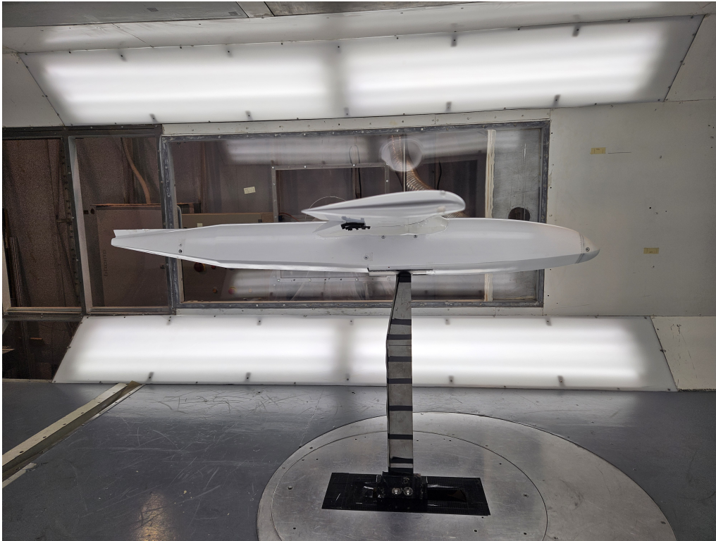
Figure 4.4: Wing-body configuration (flaps take-off)
