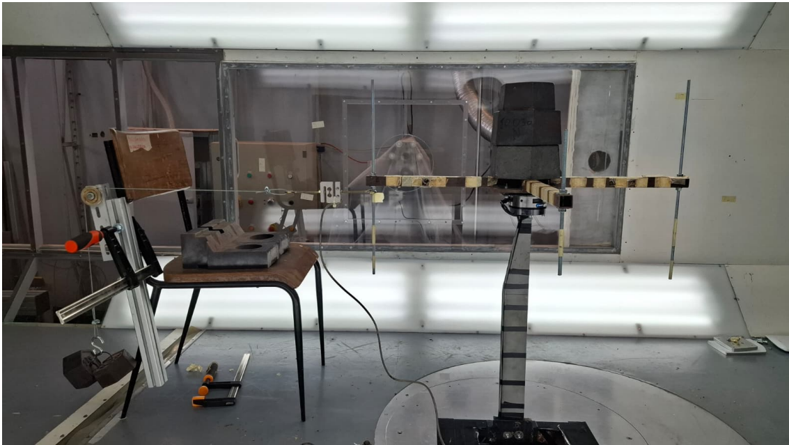
Figure 3.16: F_X calibration test.
