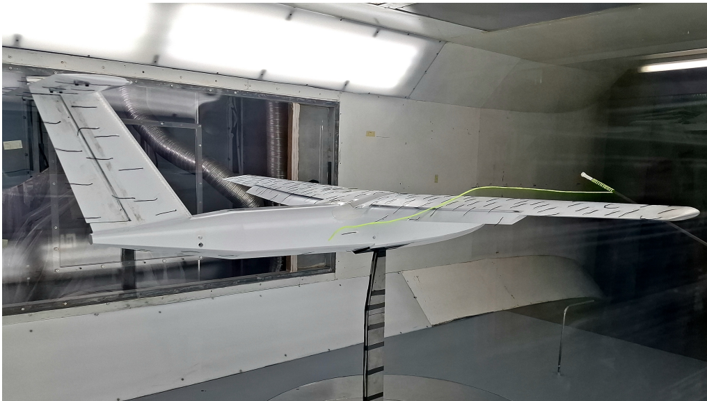
Figure 4.12: Flow visualization with flaps in take-off configuration with \delta_r = 10^\circ
