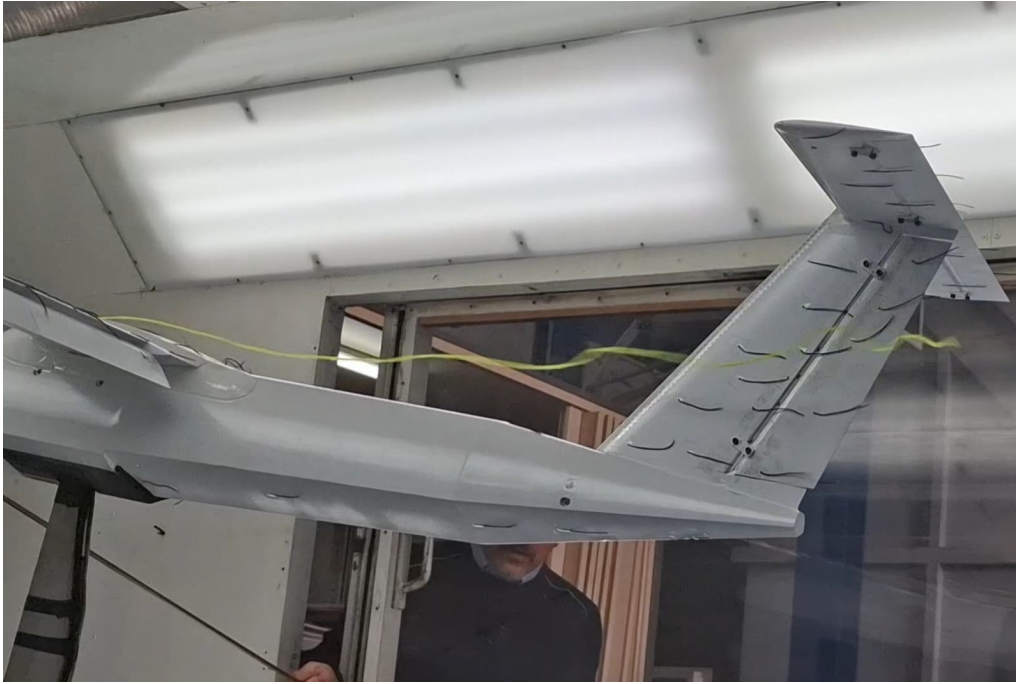
Figure 5.17: Vorticity at the vertical stabilizer due to flap vortex ( \alpha = 5^\circ , \beta = 10^\circ , flaps 30^\circ )
