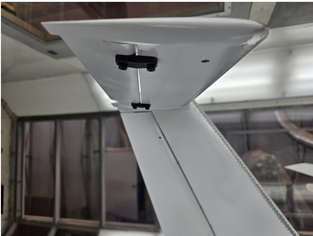
Figure 4.10: 3D printed elevator supports.
