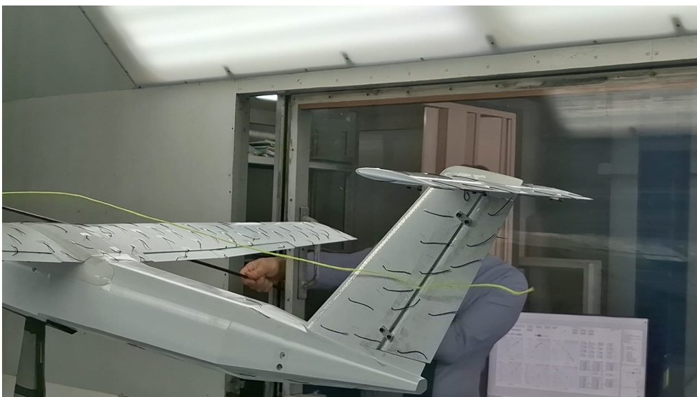
Figure 5.21: Visualization of the downwash caused by wing circulation ( \alpha = 10^\circ , \beta = 0^\circ , flaps 0^\circ )
