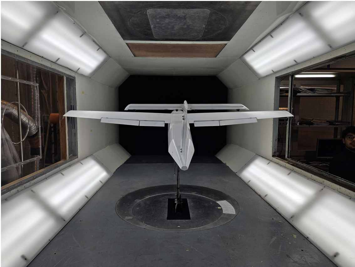
Figure 4.2: Complete model configuration, \delta_e = -10^\circ (flaps take-off)
