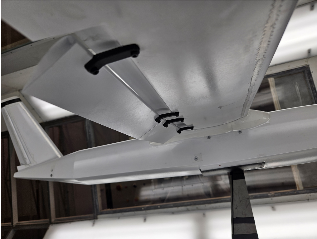
Figure 4.9: 3D printed flap supports.
