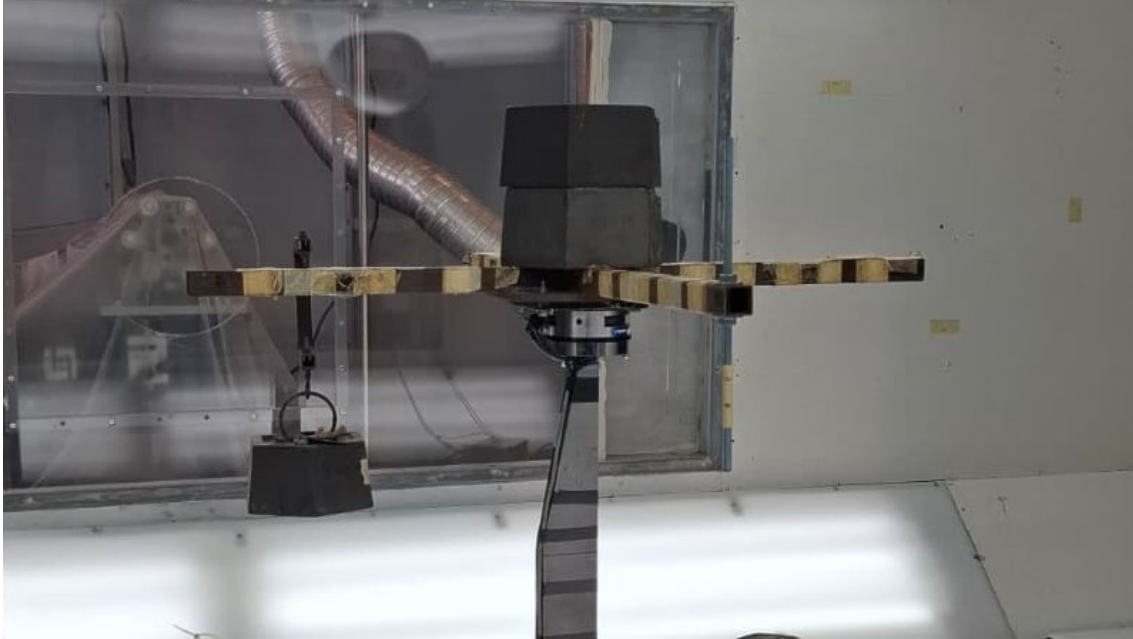
Figure 3.17: M_Y calibration test.
