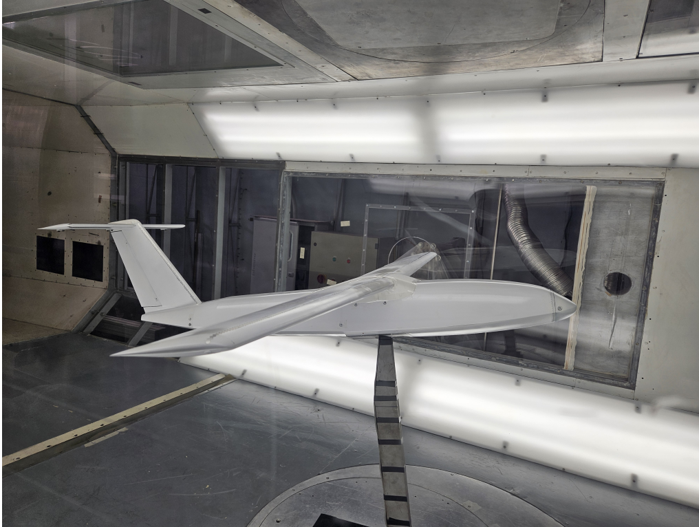
Figure 4.1: Complete model configuration (flaps cruise)
