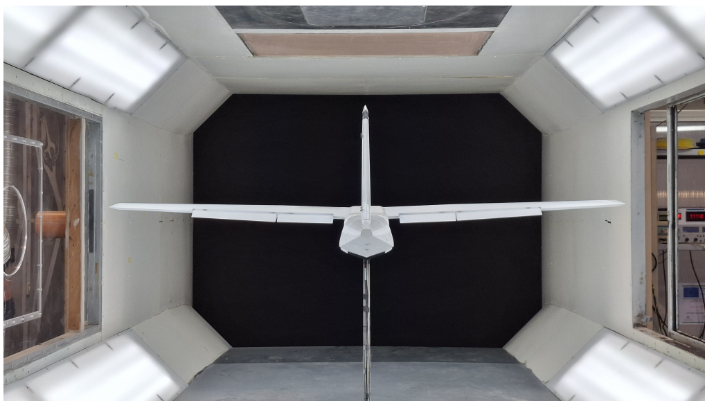
Figure 4.3: Wing-body-vertical configuration (flaps take-off)
