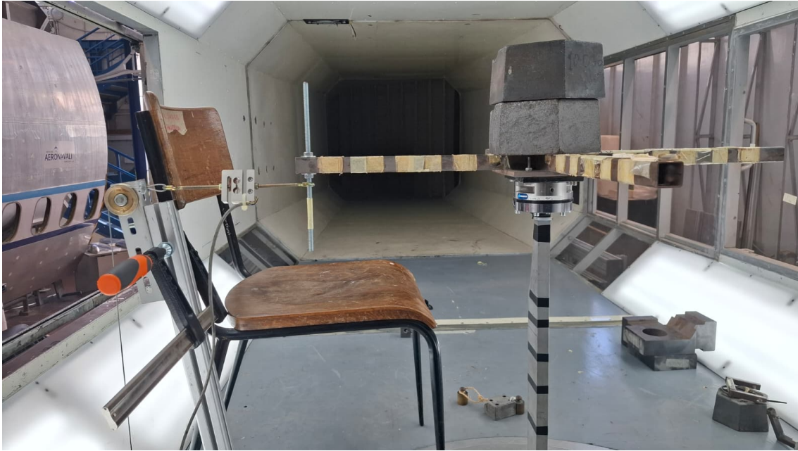
Figure 3.19: F_Y calibration test.
