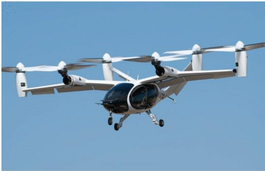
Fig. 3: Tilt-rotor Configuration Example (Joby S4-Tilt-rotor eVTOL [4]).
